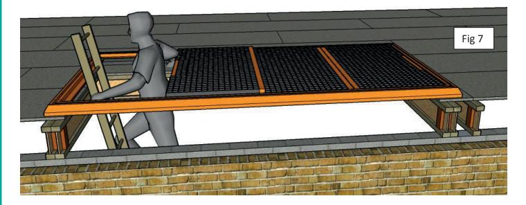
**10.** To pass large items up to the floor from below, remove whole grilles for access - always remembering to replace straight after to prevent falls through the opening.
