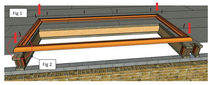
**3.** Fix the frame in position using 5mm x 100mm long screws fixed down through the 8mm diameter holes in the top of the frame down through the 16mm diameter hole in the bottom of the frame and into the chipboard decking below. See Fig 2.
