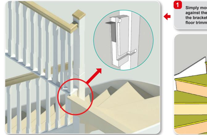
The new string section and bracket is factory fixed to the winder newel post, reducing the number of components necessary to fix on site, and speeding up assembly.
