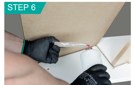
Apply PVA glue to wedges and fix in place ensuring a tight fit.
