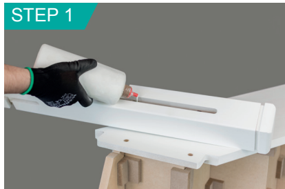
Glue mortise with PVA and fit onto string.
