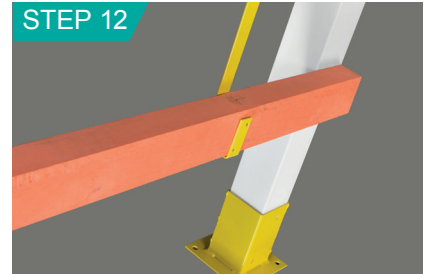
Fix intermediate rail into brackets using 4x40mm screws. Important - please ensure the minimum 80mm overlap of the newel is positioned on the side shown above
